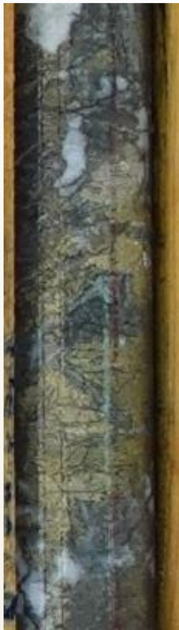
LTP-172 @ 174 m depth Strongly silicified andesitic tuff, with disseminated chalcopyrite (10%) and pyrite.
