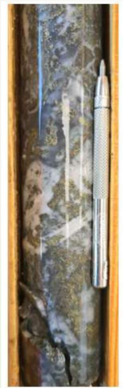
LTP-171 @ 273 m depth Strongly silicified andesitic tuff, with quartz veins and disseminated chalcopyrite (5%), sphalerite (2%) and pyrite (10%).
